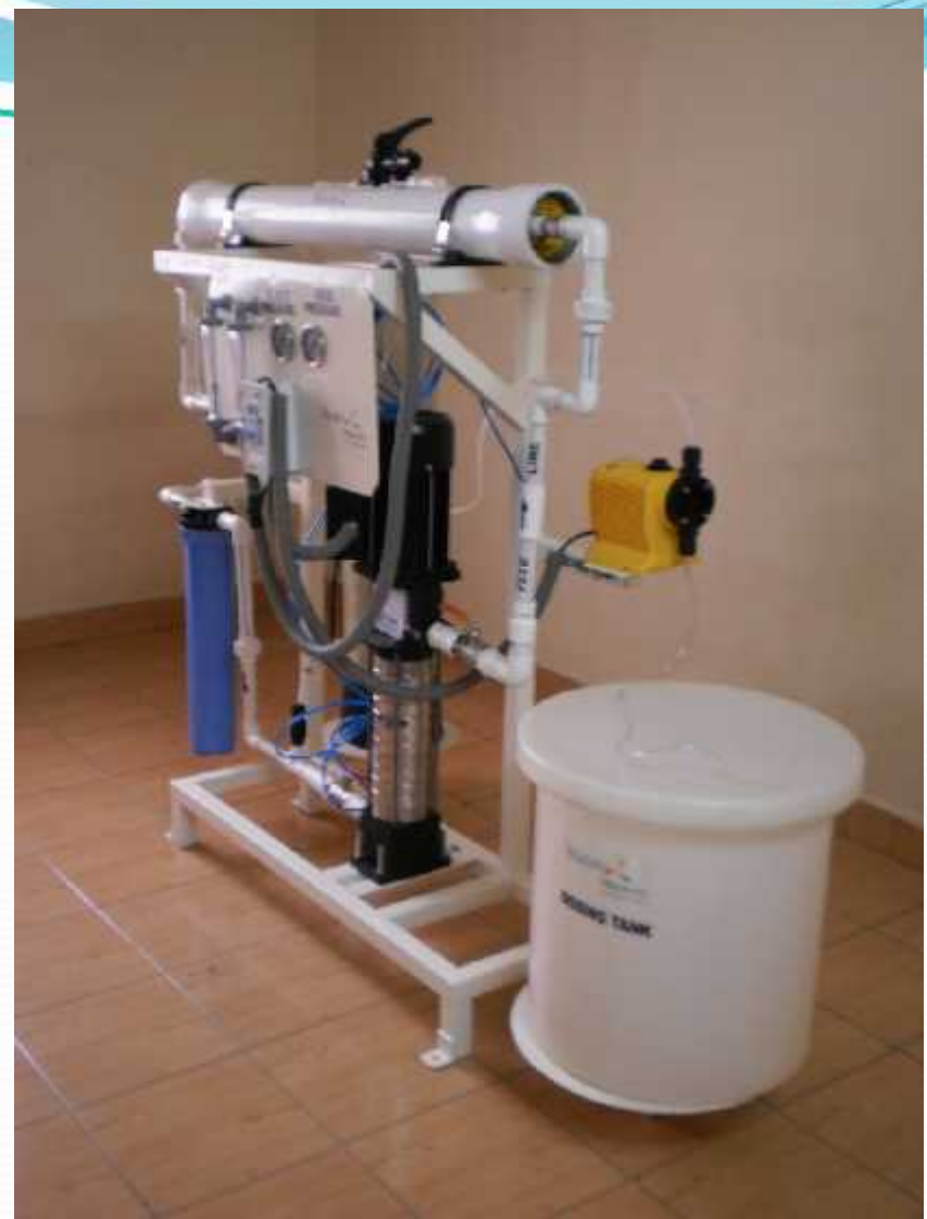
250 ltrs/hr RO Plant
